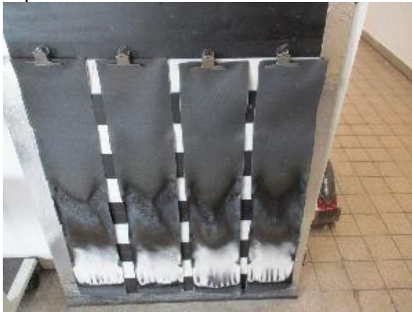
White Sample A: Material tested longitudinally in production direction
